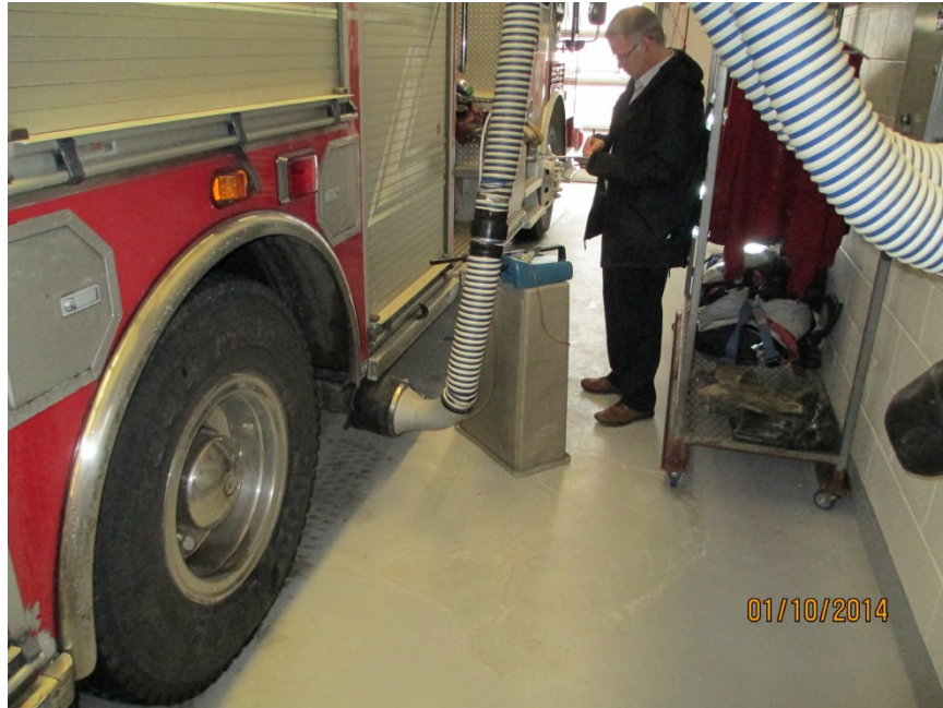
Engine 4 – Test Equipment Proximate to Exhaust Tailpipe
