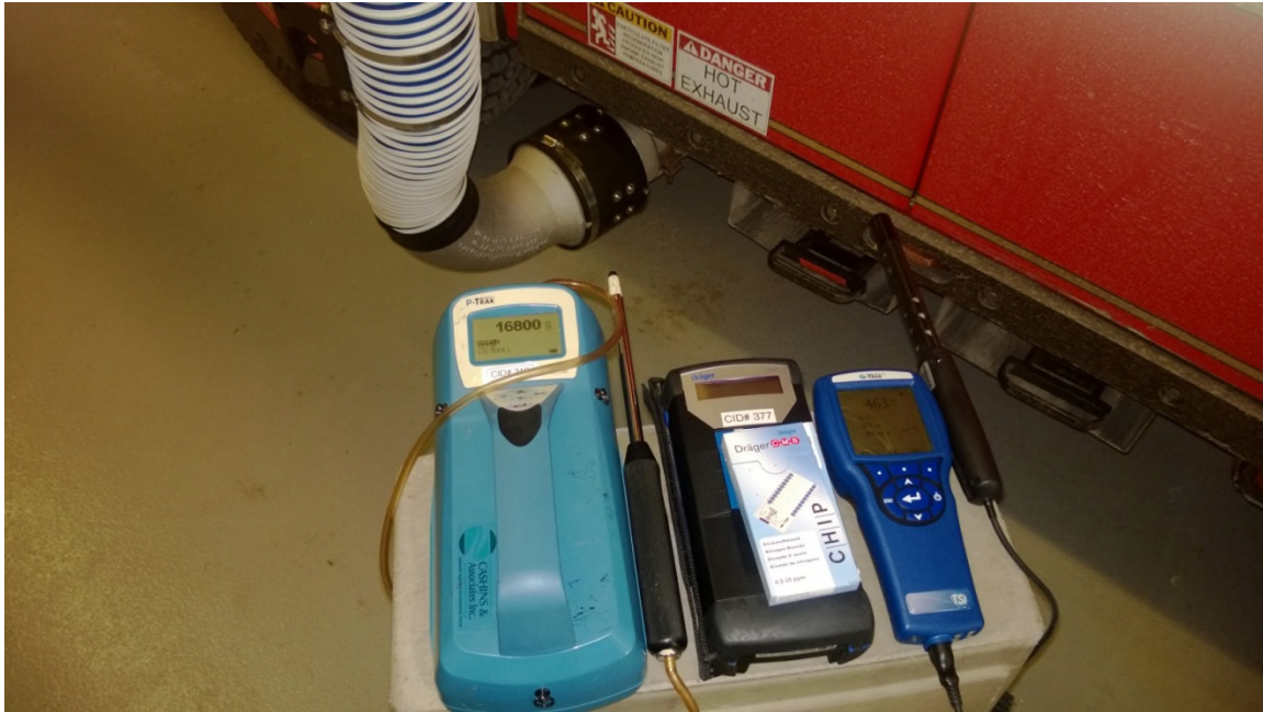
Test Instruments Setup Close to Exhaust Tailpipe
